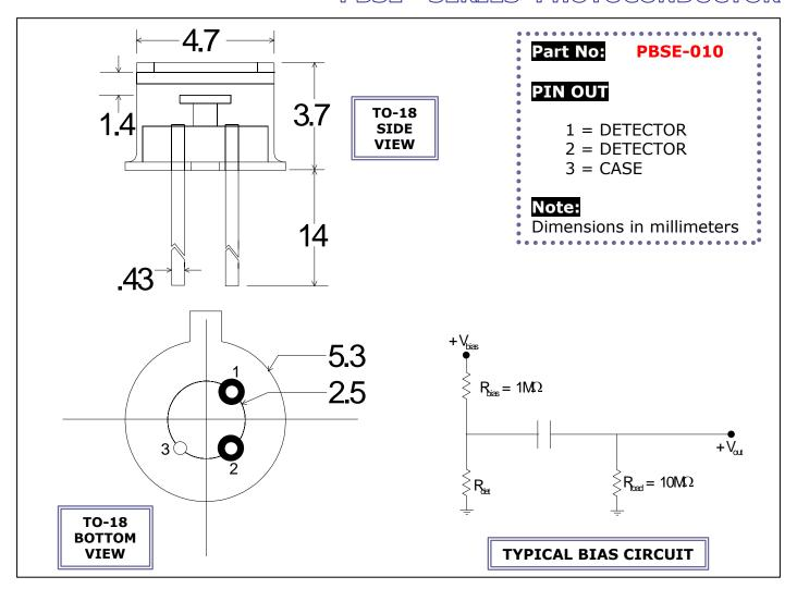
Application Note ELECTRO OPTICAL SYSTEMS offers room temperature PbSe photoconductor detectors for operation in the 1.0 - 4.5 μm spectral range. The units have state-of-the-art sensitivity and may be supported by accessories such as optical filters (longpass and bandpass), integral preamplifiers, and infrared source assemblies. These units find applications in industrial control systems, gas analyzers, thermal sensors, and general infrared instrumentation.
